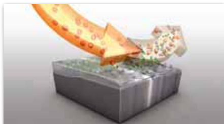
Small fillers knocked out by large particles
